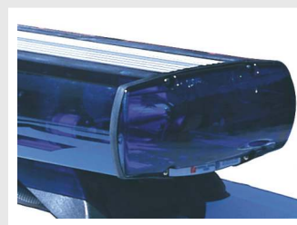
Rotating halogen priority lights
